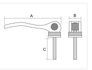
Cam lever with thread bolt, that can be used to fasten / lock parts. Often used when you need to be able to easily change or adjust a setup without tools. Often seen used on bike seats etc.
