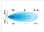
With its oval design and low height, this 10W LED worklamp is an obvious choice to sit on doorsteps on trucks or other places, where space is lacking. The worklamp has 2 powerful 5W CREE LED's, that provide up to 700 raw lumen.
