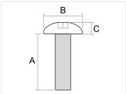
Standard bolt with M4 thread and rount unbrako head. Available in various lenghts.
