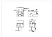
Screw terminals for through hole mounting in PCBs. 5mm pitch, 0.6mm pins. Available with 2 and 3 positions, that can be connected in a longer row.
