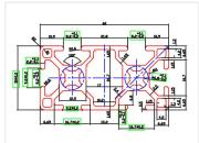
Strong 3060 profile with 2 tracks on one side. All tracks are 8 mm. The profile is produced in EU.
