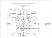
Standard 3030 profile with 8mm slot. The profile is produced in EU.
