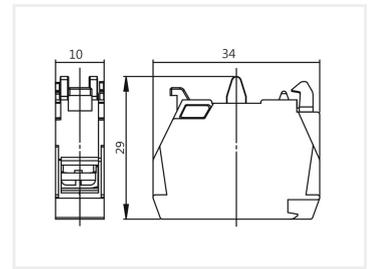
Contact for mounting in  $\varnothing 22\text{mm}$  hole, that is activated with the included keys. Available with 2 and 3 positions. A complete key-switch consists of these separate parts:
