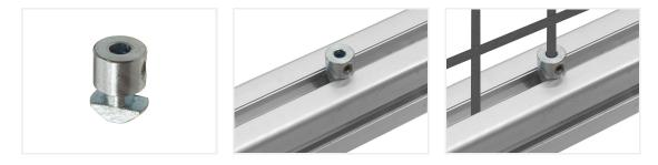
Holder for net / fence, that fits in to a series 40 profile. The holder works as a hammer bolt, but has a hole for the fence wire to fit in to, where after you fasten it with the pinol screw.
