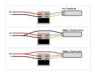
Color-changing controller for our dual color products. It can be used for both light sources with polarity inversion (2 wires), common positive and common negative (3 wires). You can also connect all types of light sources simultaneously to one controller.
