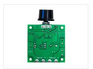
Motor-controller for small and large motors, with max 10A. Easy adjustment of speed with the dial. The dial can easily be mounted in a panel.
