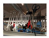
Rail with magnets, for hanging up tools and similar. 30cm or 45cm. Two or more rails can easily be put together.
