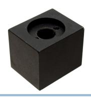
Housing in aluminium for M8 trapez nuts. Nut is mounted with 2 x M3 screws, housing is mounted with 4 x M4 threaded holes in the bottom.
