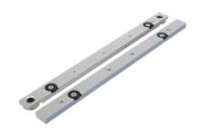
Slider that fits in the standard profiles, where it easily and freely can glide back and forth. The glider can be used for guides, fences, and jigs in machines, where you need linear motion, eg. for a sled on a table saw.
