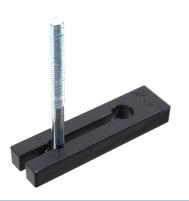
Slider in plastic, that locks itself in the profile when the bolt is fastened. This is typically used for clamps in fixtures and jigs. As it can be put directly down into the track. The special bolt needed needs to be bought separately, as it is available in various lengths.
