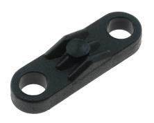
Simple clamp in plastic for strain relief of wires. The 4.4mm holes are intended for screws or M4 bolts.
