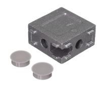
Solid 90-degree aluminium bracket for joining two 1530 profiles. The profiles with M6 threads in the center holes are bolted on to the bracket, and the included covers are placed in the holes.
