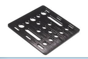
Gantry plate for v-slot tracks, that are 20mm wide, eg. 2020. og 2040. Used together with standard v-slot wheels. The plate is made of 3mm aluminium.
