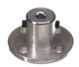
Simple coupling for DC motors, stepper motors and similar, that can be used for fastening a part to its shaft. By screwing two couplings together, it is possible to connect two axles of different diameters, eg. 3mm to 6mm.
