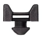
Holder for cable ties, that fit down in to series 40 tracks. Makes it easy to fasten loose cables, hoses etc. The holder is pushed down in to the track, and turned 90 degrees.
