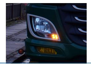
Complete set with 4 emitters for the DRL in DAF XF 2017-2021, where there as standard is white LEDs. There is a total of 8 CREE LEDs, 4 per headlight lamp. The bright LEDs have the right yellow light, similar to indicators and position lights. If you want warm white like halogen bulbs, this is also available. The xenon white variant is intended for replacing the original defective.
