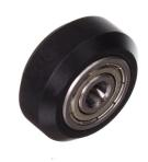
Large V-slot wheel made of Delrin, with two 625 2RS bearings. Diameter Ø24. The wheel fits standard V-slots.
