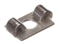
Clever clamp that is used in 90-degree joints of two profiles. The clamp is bolted on to the end of profile 1, where after your side profile 2 in over the clamp. The bolt is then fastened through profile 2 by using a access hole.
