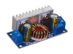
Compact step up DC boost converter with max 8A input current. The voltage can be boosted up to 42V, adjusted with the small potentiometer. Max current on the input is 8A, and 5A on the output.
