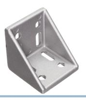
Large angle-bracket in cast aluminium for 6060 profiles in series 30, with two by two M8 mounting holes. The thickness of the bracket is 5mm.
