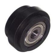
Wheel in hard plastic with a raised edge, that fits in to serie 30 and 40 tracks (8mm tracks). The wheel is used for guiding movable parts in the track of the aluminium profile. This could be a sliding door or similar. The wheel is made of durable nylon. The ball bearing ensures a smooth gliding motion, without wear.
