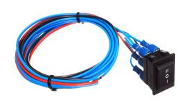
Wiring hardness with switch, that is used for driving a DC motor or actuator back and forth. As both plus and minus have to swap when driving back/forth, you cannot use a standard switch, but have to use a 2-pole switch. This switch also rests in the middle, and the motor simply stops when the switch is released.
