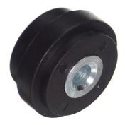
Wheel in hard plastic with a raised edge, that fits in to serie 20 tracks (6mm). The wheel is used for guiding movable parts in the track of the aluminium profile. This could be a sliding door or similar. The wheel is made of durable nylon. The bushing that is hammered in to the wheel is zinc plasted steel.
