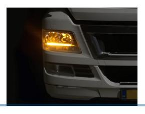
Complete kit for replaing the original white light in the DRL with yellow / amber light. The set consists of 2 boards, one for each side, and heat conductive paste to be used when mounting the boards on the original heat sinks.
