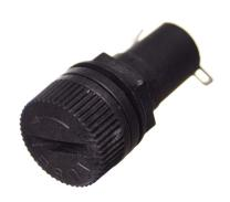
Compact fuseholder for glass fuses 20x5mm, that is mounted in a panel, eg. in a enclosure. By unscrewing the top you get direct access to the fuse, without opening the enclosure. This makes it easy to check and replace fuses.
