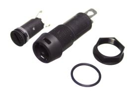
Waterproof fuseholder for 20x5mm fuses. mounted in a panel, which makes it easy to replace the fuse eg. in an enclosure, without having to open this. The top is easy screwed off with a screwdriver, where after this is easy pulled off. The fuse then sits in the top - taking the old out and putting in a new one is done easily.
