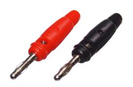
Bananaplug that can be set on a loose wire. There is a screw terminal in the plug for connection. The metal part is easily pulled out of the plastic housing.
