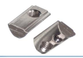
The nut can be pushed in to the series 20 profiles 6mm slot, whereafter the spring holds it in place.
