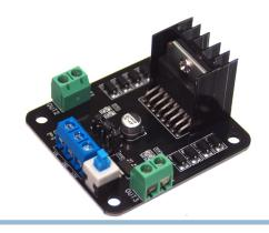
Simple and effective motor controller for 1 or 2 DC motors, with a voltage up to 24V, and max current of 2A. each channel. (Total 4A)
