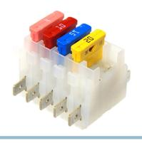
Compact fuseholder for standard ATO fuses, with 6.3 x 0.8mm cablelugs in the ends. The holder is very easy to connect. Multiple holders can be clicked together to make a simple fuse block.
