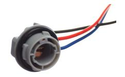
Base for BAY15D bulbs, with wires for connection. The gasket on the lamp secures a waterproof joint in a 26mm hole. There is 120mm cables in the end.
