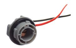
High quality BA15s base with cables, for mounting in 26mm hole. Gasket for waterproof sealing against the lamp. There is 120mm wires.
