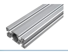
Extra strong double-width series 40 profile, typically called 4080, that eg. can be used as a basis frame in a larger constructon. There are 2 tracks on both sides, and 2 in the ends, with a total of 6 tracks, 8mm. There are also 6 holes that you can cut a thread in.
