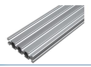
Extra wide series 20 profile, with the dimensions 20 x 80mm and 4 slots / tracks, with 6mm width. The wide profile with the many tracks makes it an advantage to use it as a table in a CNC or similar.
