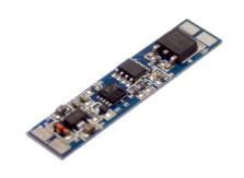
Sensor that activates when motion is sensed close by, which means it works like a motion sensor with short range. It Turns on and off the output without touch, e.g. a hand swipe close by.
