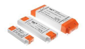
A standard transformer that is used for fixed installations. Screw-terminals on the inputs and outputs. The transformer is connected to 230V on the input and it sends 24V DC out on the output. They are primarily intended for LED installations that requires 24V.
