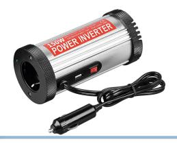
A voltage inverter that converts 12 V DC to 230 V AC, so that you can connect regular 230V appliances to a car, for example. Max power is 150W at 0.65A at 230V. There is also a standard USB plug that can be used for standard USB units. Max. USB current is 2.1A.
