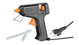
Compact and simple glue gun for 230V with 20W heating effect and up to 170 degrees. It can melt up to 16g of glue per minute. Ready for use in under 4 minutes.
