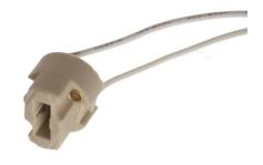
G9 socket in ceramic that fits standard G9 bulbs, both halogen and LED. There are premounted wires on the bottom.. Easily mounted with 2 screws in the base of the socket. You only need to drill two holes for the wires.
