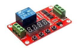
A compact and advanced timer relay with 18 different and smart features. An easy set up with the contacts and the display, where it is also possible to watch the countdown on the active function. The selected configuration is saved and activated again when the relay starts.
