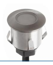
A round 35mm LED spot in stainless steel. Can be used on balconies or ceilings, creating a nice atmosphere. The spot has a hole-diameter of 32mm and a mounting depth of 36mm.
