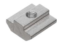
A nut that is pushed in to the end of a 40-series profile, where after it can be pushed in place. M3, M4, M5, M6 or M8 thread.
