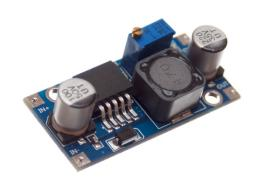
A smart compact voltage-regulator that adjusts the input voltage down to the wanted output voltage.
