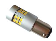
For american cars that use a single BA15YD bulb for both running lights and indicators. This one is giving a yellow light when the indicators are on.
