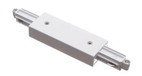
A joint for two tracks with inside screw-terminals for connecting the profiles to 230V. The two ends are pre-connected with cables and so this part can also be used as a simple joint.
