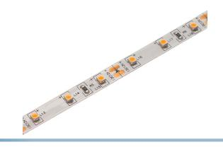
Bright LED stripes with warm white light color and with LEDs that have an extra high color rendering (RA/CRI 90+). The flexible stripes are made of many small circuits, which make it possible to cut the stripe in the desired length. You can see the length of the circuit under 'LED stripe data' below.
